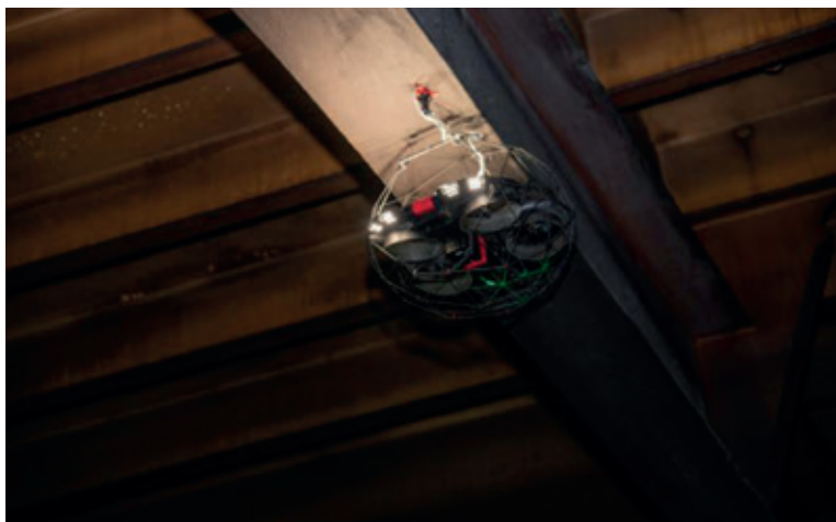
Figure 6.1. Drone taking Ultrasonic Thickness measurements (Koutsoumpas, Leontopoulos, & Zampieri, 2024)
