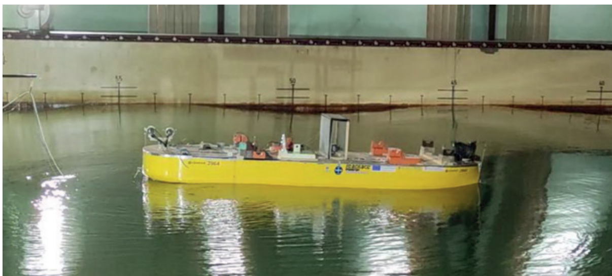
Figure 9. Seaplace DP software model tests in an eSOV (SEA-1528) at INTA CEHIPAR ship dynamics laboratory, 2024.
