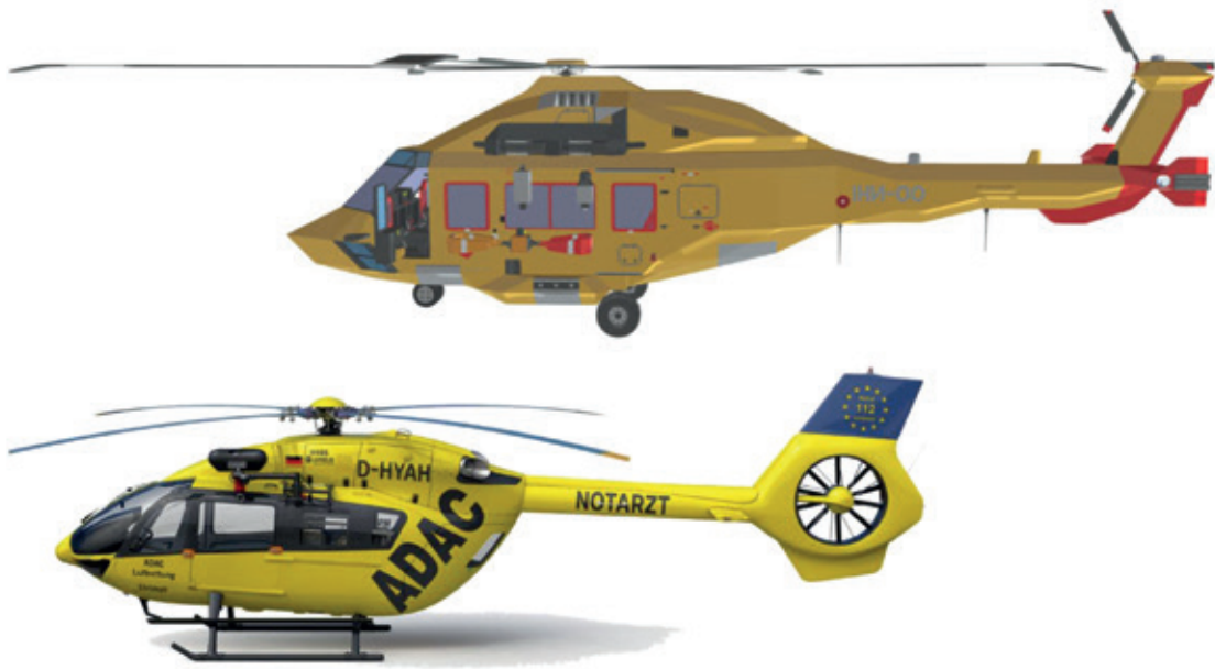
Figure 2. Side view of the H175 (up) and H145 (bottom) helicopter from Airbus
